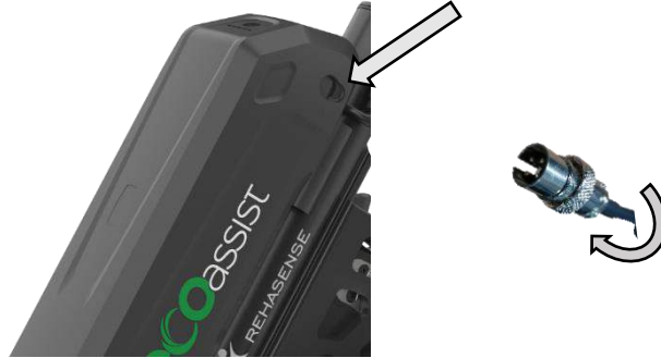
Figure 30. Battery Charging Connection.
