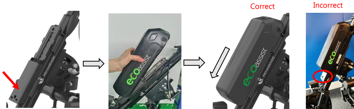
Figure 28. Inserting the Battery to the Battery Holder.
